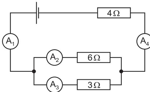
The reading of ammeter  $A_2$  is 1 A and of  $A_4$  is 3 A.
