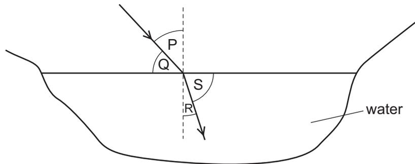
Which two angles would be correctly used in the equation  $\frac{\sin i}{\sin r} = \text{constant}$ ?
